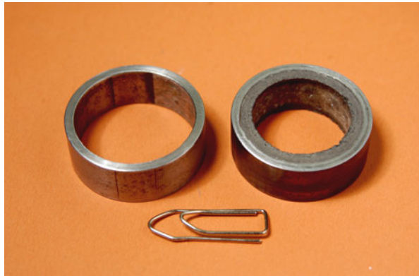
Thermal barrier lining to steel pipe
