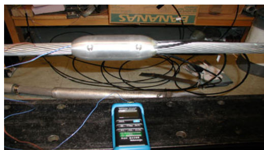
FBG sensor mounted on a simulated HT (High Tension) line
