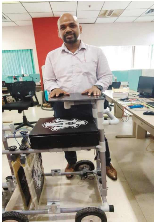
RUDI, Radar for Utility Detection & Imaging - Mr. Pragyan Prasu Patnik
