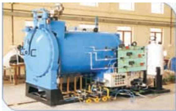
Fig: 1.56 Lab Scale Autoclave : 900mm dia x 1000mm length, Maxm. temp 200 deg C, Maxm. Pressure-7 bar(g), power 23kW.
