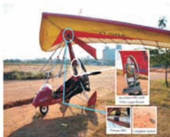
Fig: 1.54 Integration of autopilot hardware with data logger to the Powered Hang Glider.
