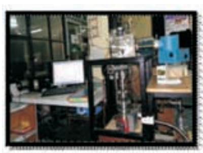
Fig. 1.79 Developed Large Volume Penning plasma discharge (LVPPD) source for VUV-spectrometer-detector-system calibration at CSIR-CEERI
