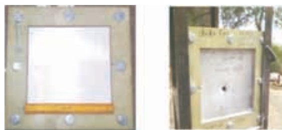
Fig: 1.42b (L) Alumina Ceramic composite armour test plate (500 X 500 X 50) mm³ of weight = 29.7 kgs and (R) Testing of ceramic armour panel at
