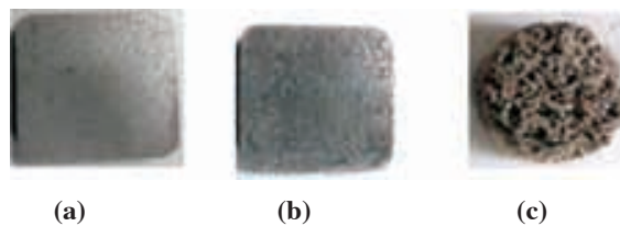
Fig:1. 38 Ti-foams of varying porosities : (a) 65%, (b) 75% and (c) 85%
