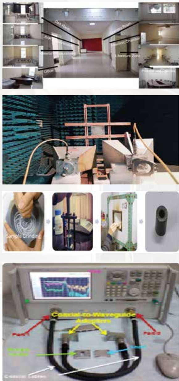
Fig . 6 (a) CRTDH Center at IIT Roorkee (b) Measurement setup for sample preparation (c) Bistatic measurement setup
