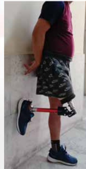
Fig. 2 Patient specific prosthetic polycentric knee joint and socket for trans femoral amputees
