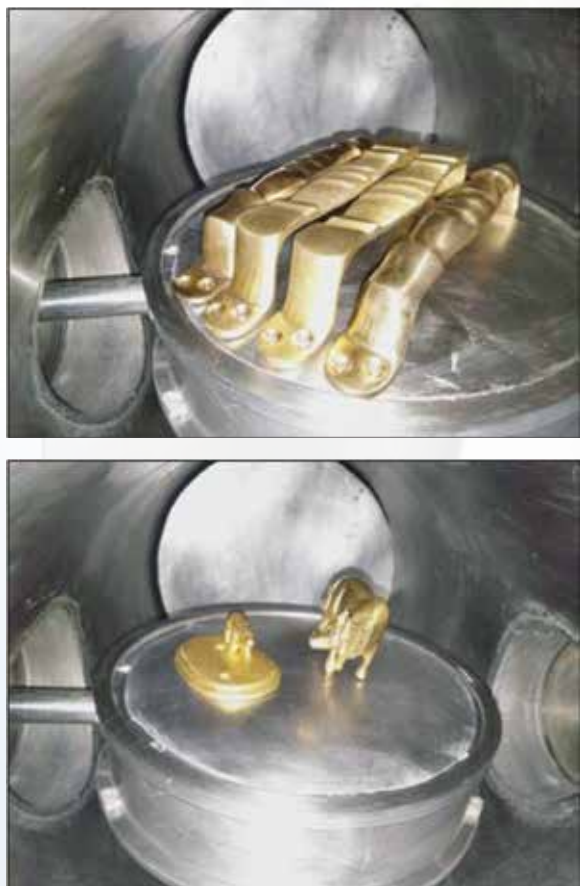
Fig 8: Coated copper alloys using radio-frequency plasma technology
