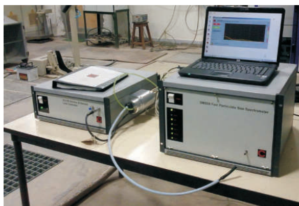
Fig. DMS is the only available equipment which can be used for on-road particle size distribution measurement
