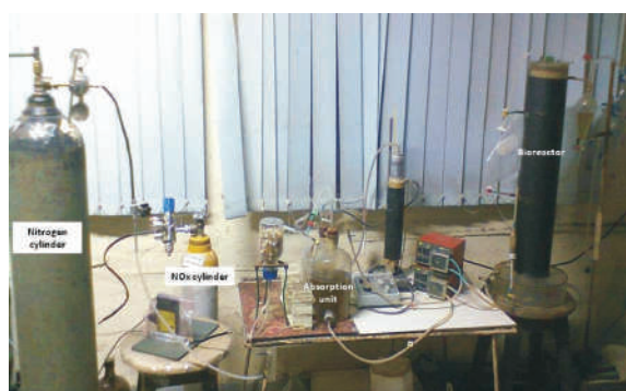
Fig. Bench Scale reactor system for chemo-biochemical deNO x ing
