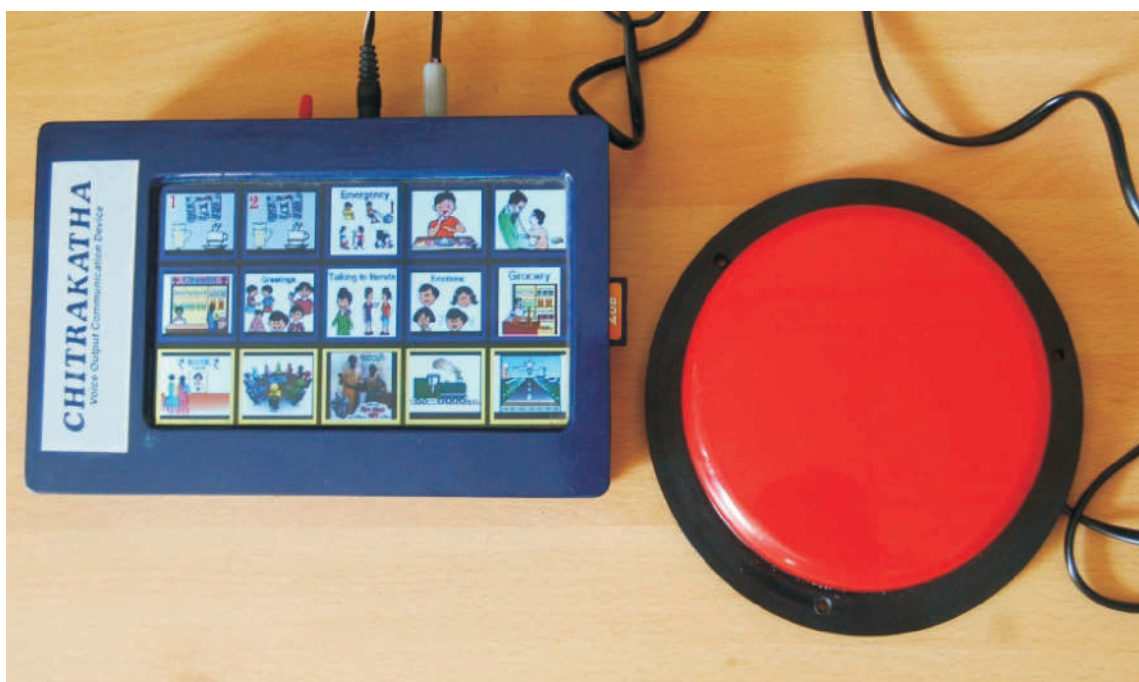
Multi-layer, Scannable, Voice Output Communication Aid and Special Access Switches by Er. Shamit Patra, TUC, IIT, Kharagpur
