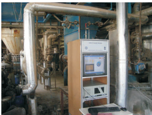
Fig. NIRS based on-line instrument for quality assessment in edible oil industry
