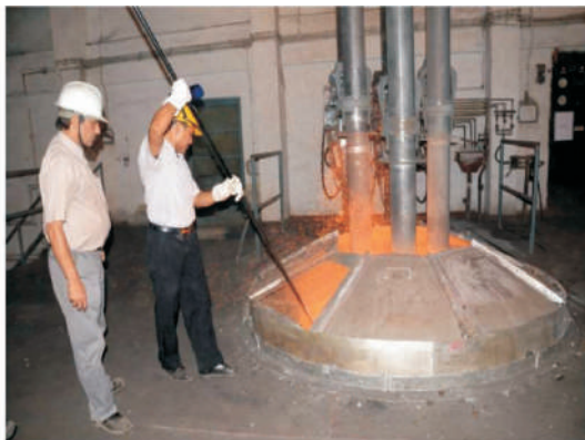
Fig. Pilot Scale submerged arc furnace operation
