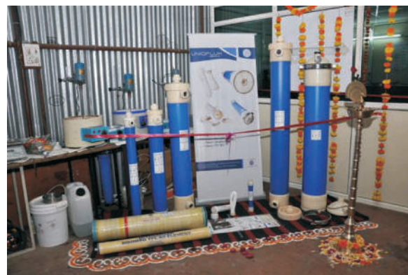
Fig. HF membrane modules based on CSIR-CSMCRI knowhow prepared by M/s Uniqflux
