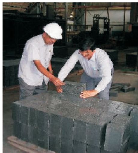
Fig. Upscaling of MgO-C Brick at Vizag Steel with modified Technology of CSIR-CGCRI.
