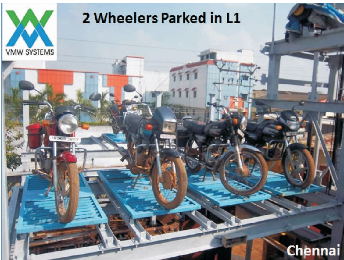
Multi-level Automatic Two Wheeler Parking
