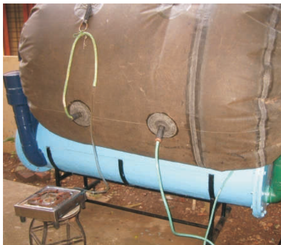
Fig. Household Wastes Digester cum Biogas plant
