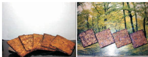
Fig. Prototypes of Thermal Insulation Sheets from Forest Dried Leaves Waste
