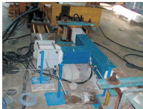
Fig. Test set for cyclic test on beam-column joint
