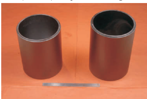
Fig. Photographs of IGCAR's graphite crucibles coated with PyC coating
