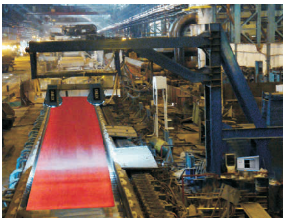
Fig. Online surface inspection module for hot rolled steel strips
