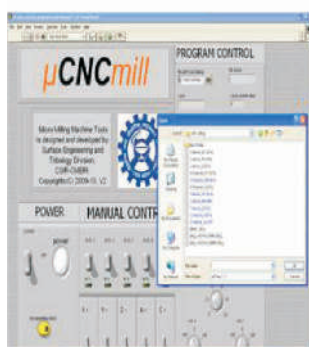
Fig. GUI of \mu CNC mill Control System
