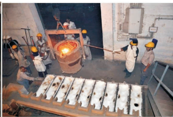
Fig. Metal tapping from submerged arc furnace
