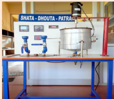
Figure 5: Automated reactor vessel to produce bio-modified ghee
