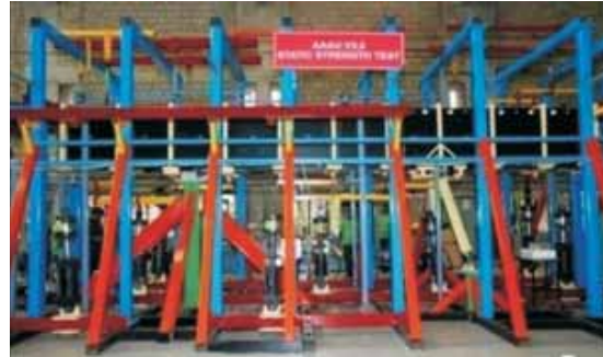
Static structural strength test setup for AAAU
