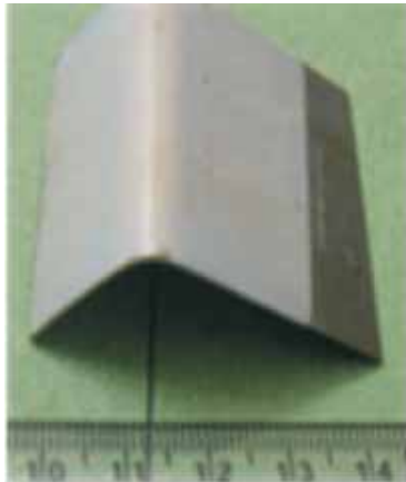
TiO 2 coating on steel developed- 1200 hrs. salt spray test, withstand 500°C and 90 degree bend test
