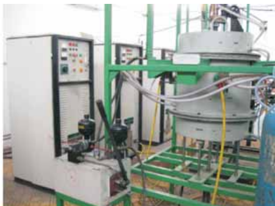
50 kW arc plasma reactor
