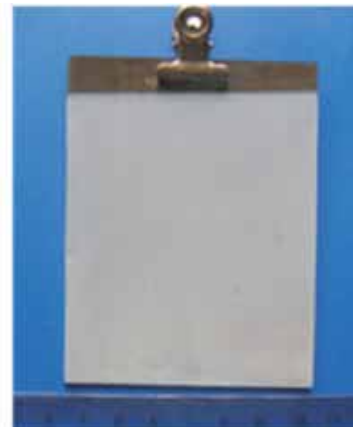
TiO 2 coating on steel developed- 1200 hrs. salt spray test, withstand 500°C and 90 degree bend test
