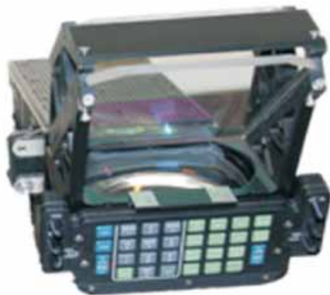
Head-up Display System for HJT-36 Aircraft
