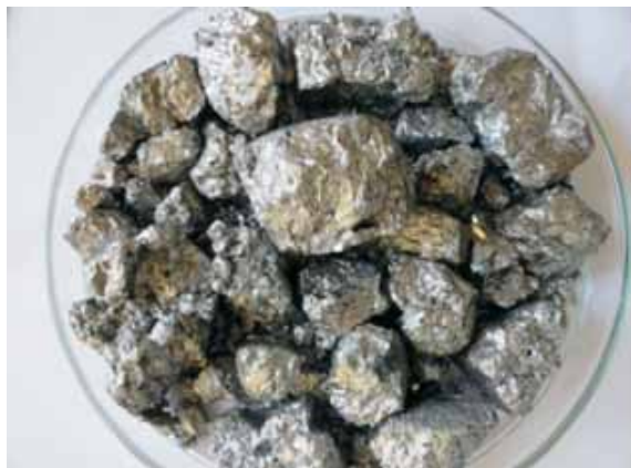
Molybdenum, tungsten and nickel rich alloy and alumina rich slag obtained from catalyst residue by smelting
