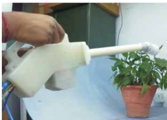
Prototype of Air-Assisted electrostatic sprayer for agricultural applications
