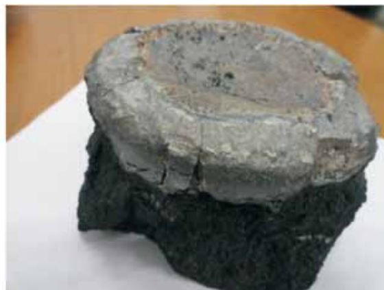
Molybdenum, tungsten and nickel rich alloy and alumina rich slag obtained from catalyst residue by smelting
